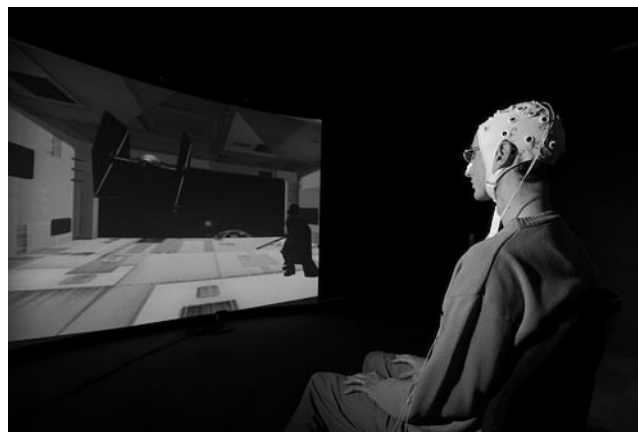
Figure 10. The use-the-force application. In this application, the user can lift a virtual spaceship by performing real or imagined foot movements. (©CNRS Photothèque/Hubert Raguét)
